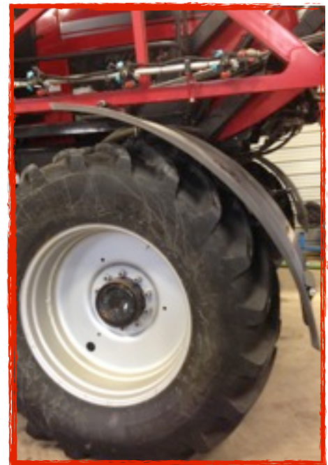
Left: Patented bolt-latch fender extension. Above: Side profile of fender extension.
