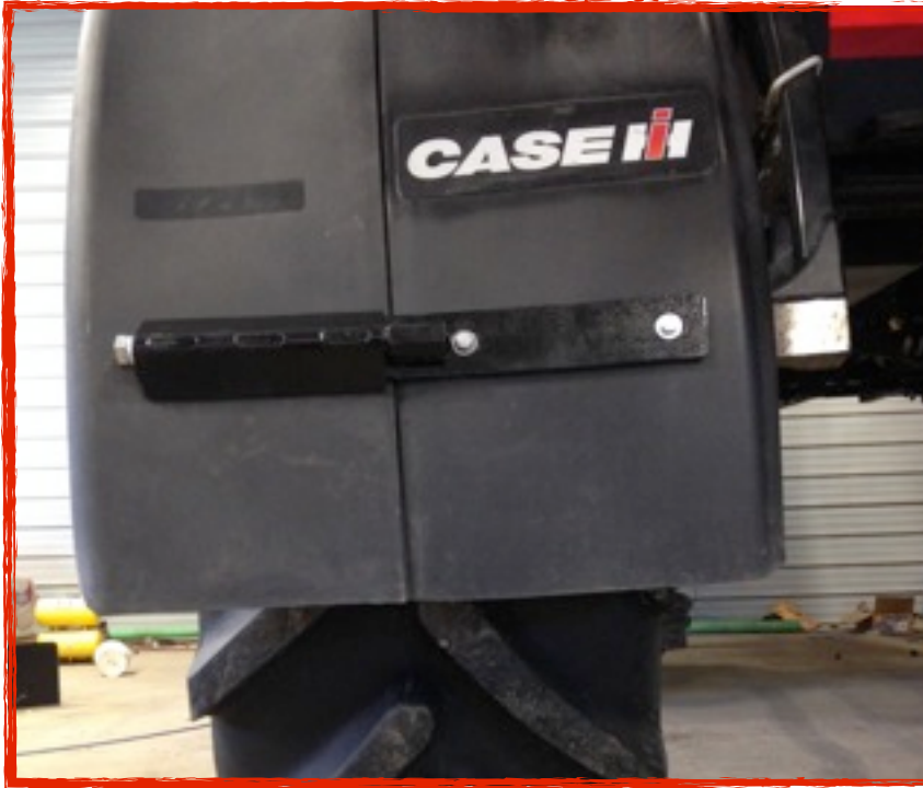
Left: Patented bolt-latch fender extension. Above: Side profile of fender extension.
